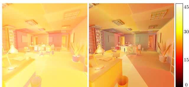
Figure 8: Heat map illustrating the reduction of the number of accessed nodes when continuing light transport paths from the node of intersection (right) instead of starting traversal from the root node (left). As close occlusions are found faster, the image on the right resembles an ambient occlusion rendering.
